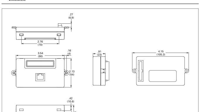
Figure 13. HMICENT Ethernet Expansion Module — Approximate Dimensions in Inches (mm)
